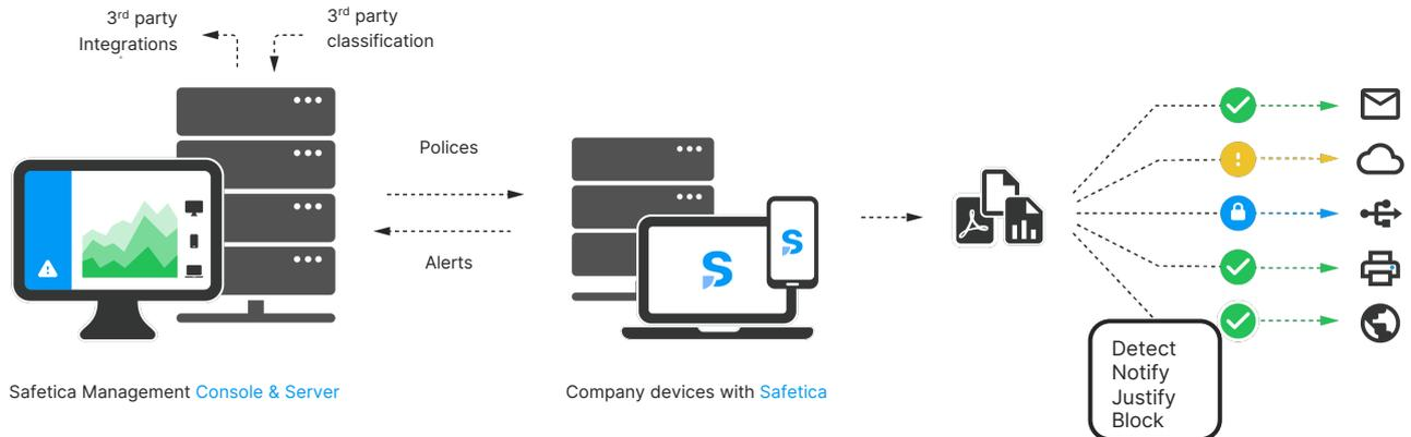
The physical or virtual server runs a database with endpoint activity and security records. The Safetica Management Console enables admins to manage security policies and display the collected information.
